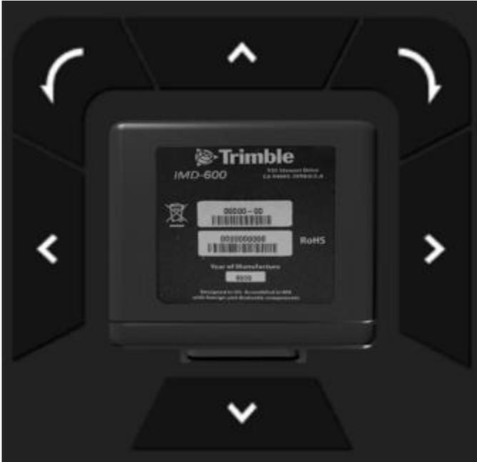
IMD Orientation - This allows the user to describe how you have mounted the IMD. In the depiction, the nose of the vehicle is towards the top.
